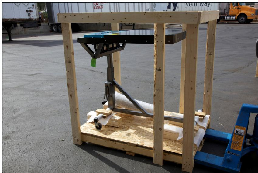
2. The box inside of the plastic wrapping contains the quartz heating elements. Handle the package with care, and don't touch the elements with bare hands. Use a clean cloth to handle the elements.
